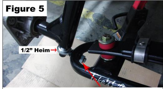
Jam nut also called half nut on inside of bottom a-arm
