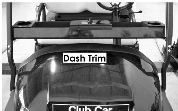
Tech Tip: use a clamp on each side for clamping the brackets into place. Set tray on and center everything then mark your holes before drilling.
