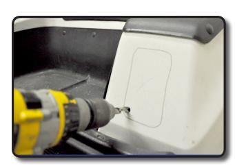
Insert tail light and attach tail light to cart using provided hardware.
