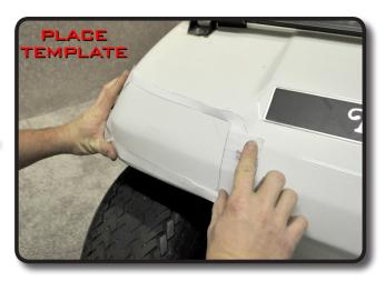
Draw the inside of the template out with a writing utensil. Next drill a pilot hole so you will have a starting point to begin cutting.
