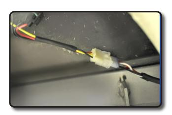
Secure remaining harness under cowl using provided ties.
