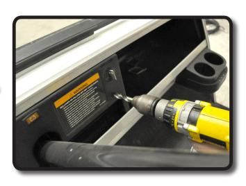
Feed threaded end of switch through the dash where the hole was drilled. Tighten and attach harness as shown.
