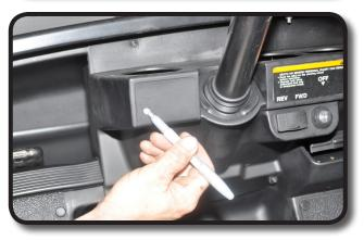
Use a 15/32" drill bit and drill at location marked in Step 2.
