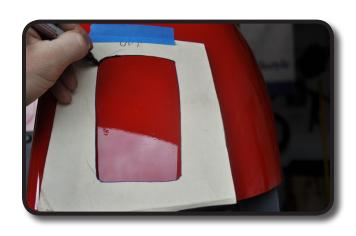
Drill a pilot hole and cut, again staying to the INSIDE or on the mark.
