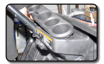
Locate a place on the dashboard to mount the switch. We recommend using the location shown as it does not interfere with the cup holder when reinstalled and also allows you to easily route the wiring harness.
