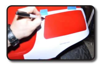
Drill pilot holes on the INSIDE of the marks as shown.
