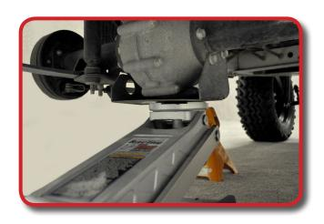
Using a 5/8" Socket remove the driver side U-Bolts. Once the U-Bolts are removed you can remove the lower bushing and shock using a 9/16" Socket. Retain shock hardware. Discard U-Bolts and nuts.
