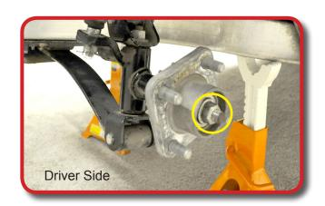
Using a 1/2" Socket remove bolt from shock and discard push shock up and out of the way.
