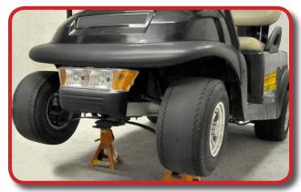
Detach front bumper by removing the two factory bolts closest to the edge of the frame. Retain bumper and hardware.
