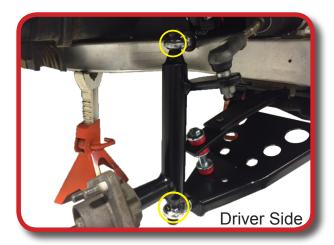
Reattach tie rod to spindles using retained castle nut and cotter pin from step 6.
