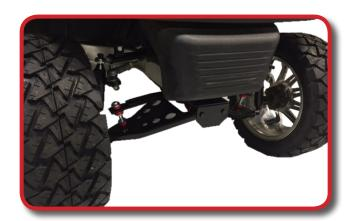
Chock front wheels, then disengage parking brake. Lift rear of cart and support with jack stands under the frame. Remove rear wheels. Leave jack in place under axle and motor assembly.
