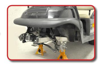
Using a 21mm Socket remove and retain hub and flange nut. Repeat on passenger side.
