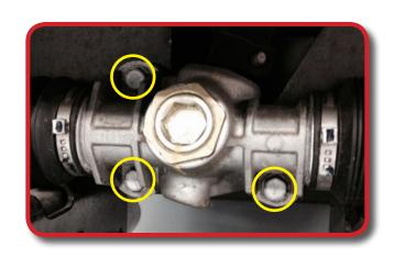
Using a 1/2" Socket remove factory A-Arms. Retain hardware.
