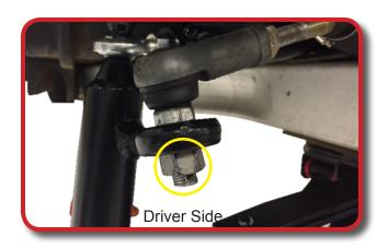
Using a 13mm Socket and Wrench Reattach shock to A-Arm using the two 8x50mm Hex bolt, four locknut.
