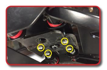
Note: Before attaching spindles, adjust heim joints so there is approximatly 1/4" of thread showing.
