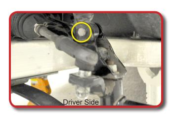
Remove and retain the cotter pin from the tie rod end, using an 18mm Socket and an 11/16" Wrench. Remove nut from tie rod.
