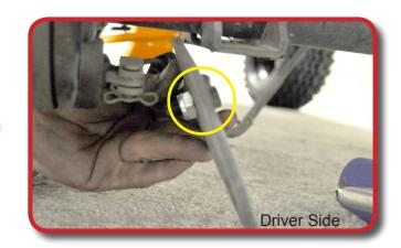
Route U-Bolt through Shock mounting plate around axle and through factory lower bracket making sure alignment bolt attached in step 27 fits properly in axle. Using a 17mm socket tighten U-Bolt evenly to ensure proper alignment.
