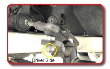
Using 1/2" Socket remove factory spindle by removing bolts as shown in picture.
