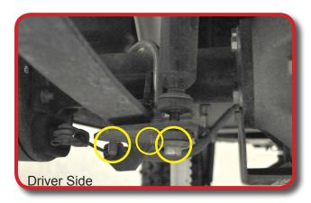
Using a 10mm socket and 13mm wrench remove hardware from rear leaf spring mount. Retain hardware.
