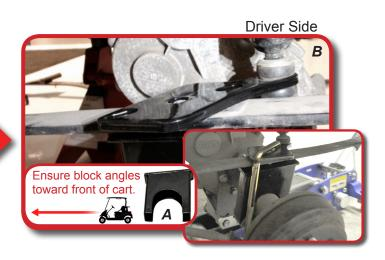
Using 6mm Allen Wrench and 13mm Wrench attach bolt from hardware pack through the factory lower bracket as shown. This bolt does not serve as a fastener, its only purpose is to provide the proper placement of the bracket under axle. Tighten hardware.
