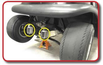
Using a 3/4" Socket remove front wheels.
