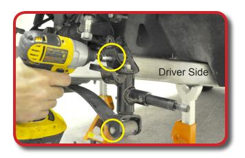
Using a 1/2" Socket remove spring plate and leaf spring. Retain spring plate, discard hardware and spring.
