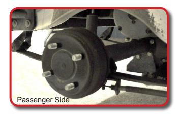
Using a 5/8" Socket loosen the U-Bolts on the passenger side.
