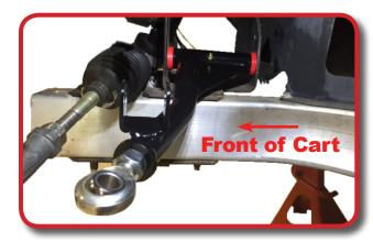
Using hardware retained in Step 9 reattach rack and pinion.
