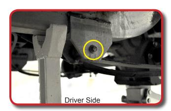
Use jack to lower axle and motor assembly. Reinstall leaf spring on top of axle using hardware retained from Steps 23 and 24.
