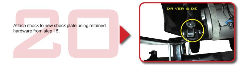
Repeat steps 15-20 on passenger's side. Use jack to lower axle and motor assembly as needed. Once complete, install new wheels, lower cart and proceed with alignment as shown on next page.
