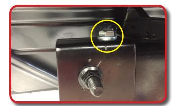
Additionally secure shock mounting bracket using factory shock and bumper hardware as shown. Tighten all hardware.
