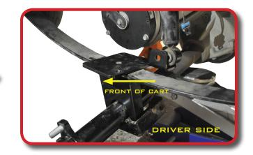
Route supplied U-Bolt down through the top of the Rear Shock Mounting Plate to the bottom factory bracket. Be sure that all alignment bolts are in correct position to keep axle straight. Using a 17mm socket tighten U-bolt evenly to ensure proper alignment.
