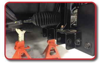
Mount factory A-Arms to main bracket using the 10mm x 80mm bolts and hardware.
