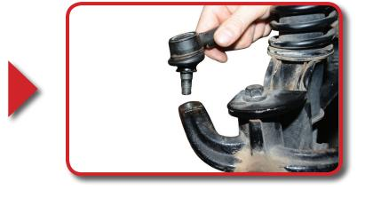
Using a 15mm socket and wrench remove hardware from top of the shock and from the lower control arm. Remove factory suspension assembly from cart. Retain hardware (factory suspension will not be reused).
