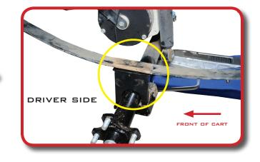
Using the supplied hardware, place bolt on factory bracket as shown and tighten.
