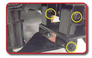
Attach factory shock to shock mount bracket using 10mm x 65mm bolts and hardware as shown.
