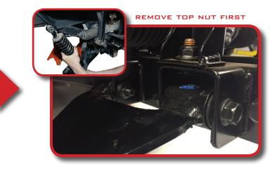
Attach shock mounting bracket to top of upper frame using 10mm x 25mm bolts as shown. DO NOT tighten until after next step.
