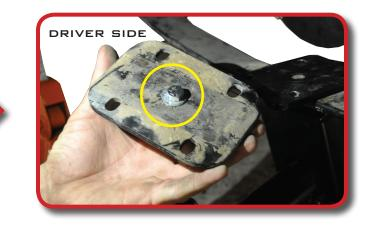
Attach Rear Shock Mounting Plate to top of the spring as shown.
