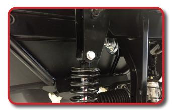
Attach new spindles to factory spindle mount using factory hardware, repeat on opposite side.
