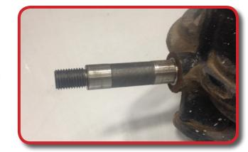
Using a 17mm socket remove cotter pin and castle nut from tie rod and remove the tie rod from the spindle. Retain hardware.
