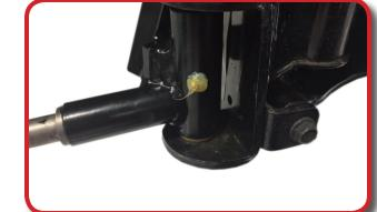
Using 17mm socket attach steering rack to new spindles using retained hardware from STEP 4 Repeat process on other side.
