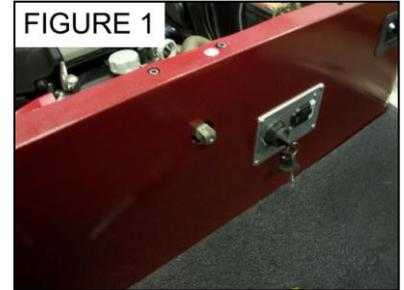
1. Place the cart in neutral and remove the stock shifter from the cart as shown in Figure 1. Save the stock screw for installing Jake's new sport shifter.
